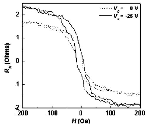
FIG. 3. Hall resistance at a given gate voltage of  $V_g = 0$  and  $-25$  V as a function of the magnetic field applied in the direction of the ferromagnetic film axis.
