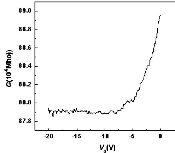
FIG. 2. Conductance of the device as a function of gate voltage.
