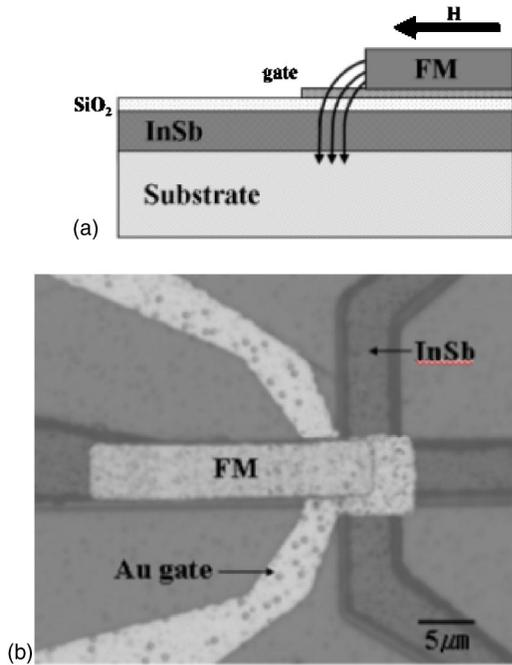
FIG. 1. A schematic diagram of a cross-section view of the gate-controlled InSb Hall device (a) and an optical micrograph of the fabricated device (b).
