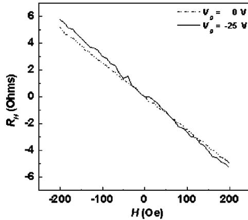
FIG. 4. Hall resistance at  $V_g=0$  and  $-25$  V as a function of the magnetic field applied in the direction perpendicular to the device surface.
