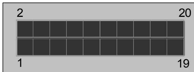
Figure 1-3 GPI/Serial Connector Pinouts
