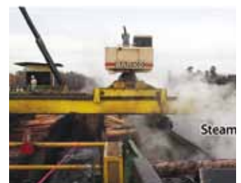
Operators cannot see through the steam cloud caused by condensation in cooler air temperatures.
