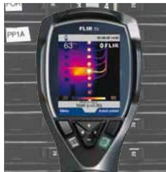
FLIR i5, temperature in 6,400 spots
